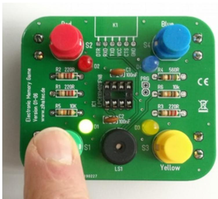
*If one or more LEDs not shine, you have to check the assembly direction (cathode/anode) of these LEDs. Furthermore check the soldering of the LED, corresponding resistor and button.*
