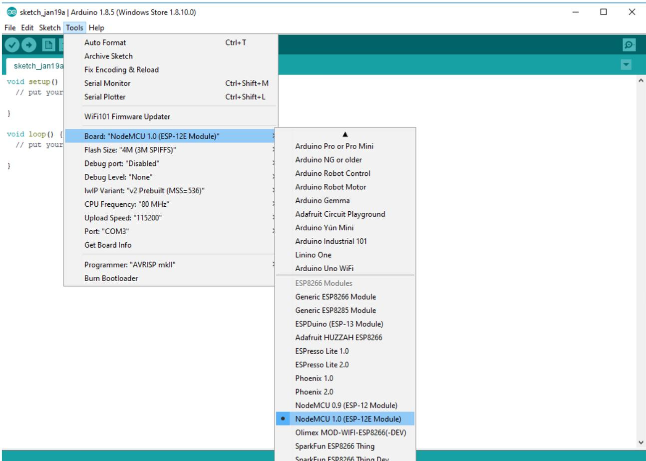
For the Wemos D1 Mini you have to choose **WeMos D1 R2 & mini**. Set the CPU frequency to 80MHz, Flash Size to „4M (3M SPIFFS)“, the baud rate of your choice and the COM port.
